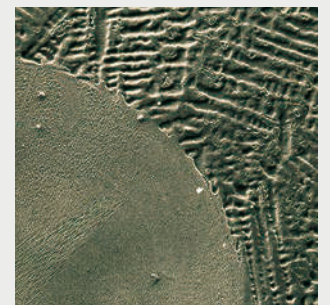
Laser weld without any cracks in a carbon-free CoCrMo alloy
