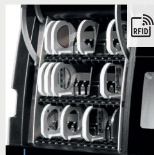
Integrated and RFID-controlled blank tank
