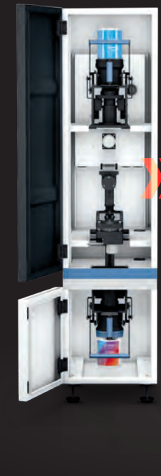
Sieving unit for powder recycling
