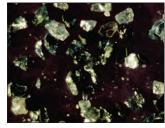
Silicon carbide microparticles contained in Opalustre slurry.
